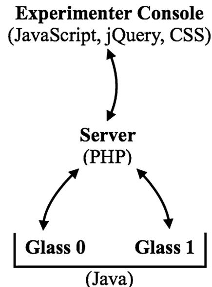
**Fig. 2** PsyGlass framework flow and the programming and/or markup languages of each component (listed in parentheses). In the experimenter console's current form, the researcher can use it to update visual displays on one or more connected Glass devices while collecting accelerometer data from each
