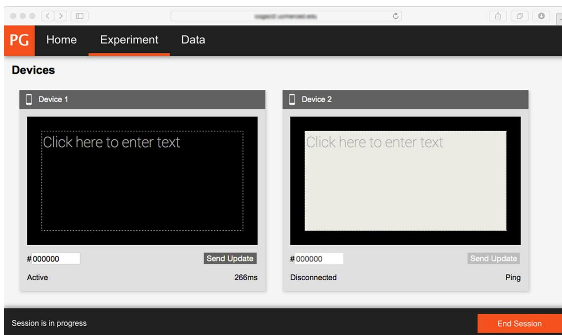
**Fig. 3** PsyGlass experimenter console. From here, the experimenter can manage the connection between the connected Google Glass device(s) and the server, initiate data collection sessions, and update the Glass screen(s) with text and/or color
